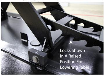
Note: When lift is not in fully lowered position, it is recommended that the nearest lock position be used.
